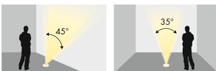
Asymmetrische Linse 45°/35° / Asymmetrical lens 45°/35°
