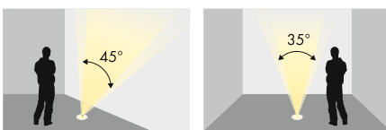
Asymmetrische Linse 45°/35° / Asymmetrical lens 45°/35°
