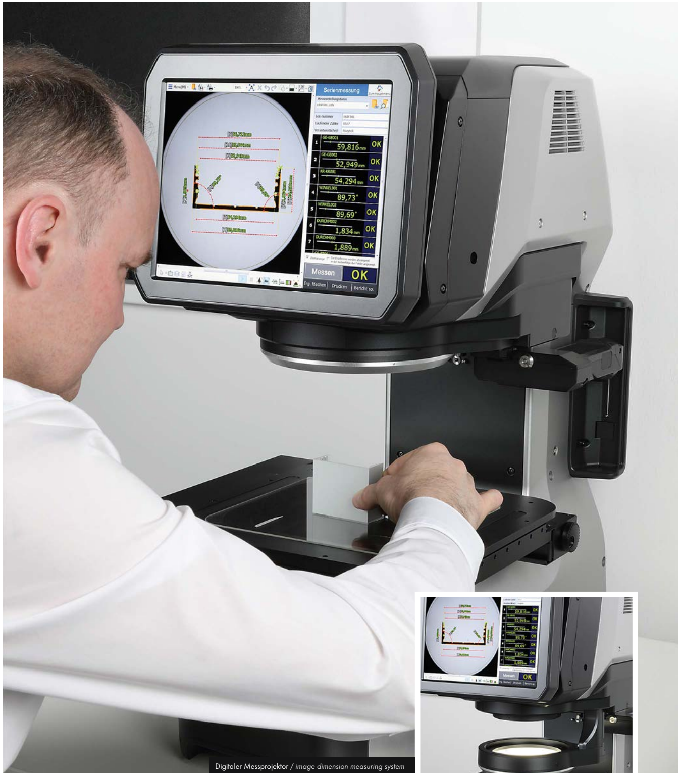
Digitaler Messprojektor / image dimension measuring system
