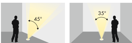
Asymmetrische Linse 45°/35° / Asymmetrical lens 45°/35°
